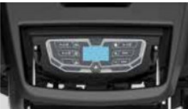
New control panel suitable for FMS system with brush pressure adjustment
